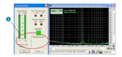
7. If the recording volume level is not enough, check and make the WAVE and Master volume have been at the maximum level; Instead, if the recording volume level is too high, lower the WAVE and Master volume gradually until the level is ok.
