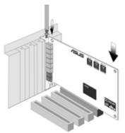
2. Secure the audio card bracket to the back of your computer with the screw that you removed. Refer to section 3.1.
